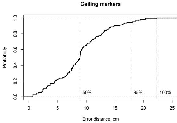
Fig. 3: HIPS positioning performance using ceiling markers (all participants).
