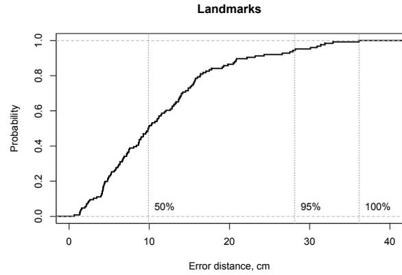
Fig. 5: HIPS positioning performance using environmental landmarks (all participants).
