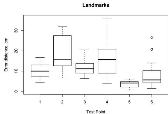
Fig. 6: Localization error of landmark-based HIPS in different test points.
