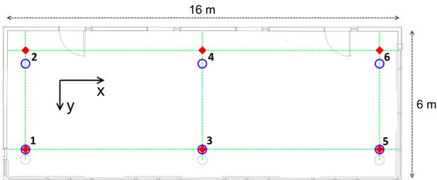
Fig. 2: Testbed layout. Floor and ceiling markers are labeled with blue circles. The environmental references are represented by the green lines aligned with pillars ( $x$ -landmarks) and window frames ( $y$ -landmarks); corresponding test points are labeled by red diamonds. Please note that test points 2, 4 and 6 are different for the marker-based and landmark-based scenarios.
